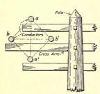
Fig. 102.—Arrangement of twophase conductors on cross arms.
